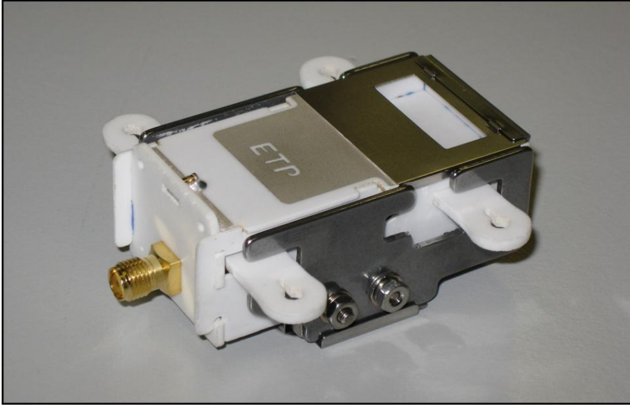
Figure 8. Photo of the new DM430 compact magnetic TOF detector. The SMA signal connector gives an indication of size.
