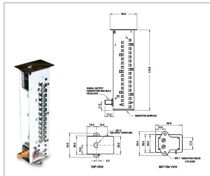
Photograph of a DM169 prototype Scaling Pulse Detector and schematic showing mechanical detail.
