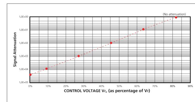
Figure 3. Attenuation of the measured output pulse rate of a DM169 Scaling pulse Detector as a function of the control voltage, Vc.
