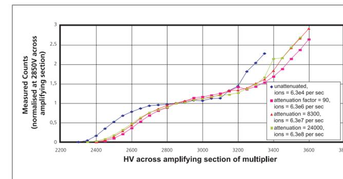
Figure 2. Plateau curves obtained at attenuation factors of ~1, ~90, ~8300 and ~24000. Datas were recorded with a discriminator level of 1.0mV.
