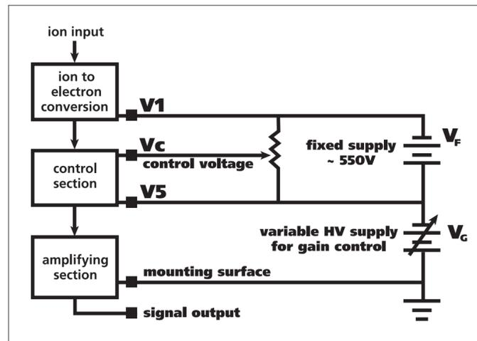
Figure 1. Schematic diagram of multiplier operation.
