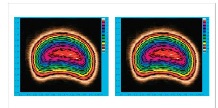
Figure 4. A contour plot of the spatial sensitivity within the aperture of a DM169 Scaling Pulse Detector (dark lines are 10% sensitivity contours). The aperture scan was produced by rastering a ~2mm diameter beam of air ions across the multiplier aperture. Little change is seen between the attenuated and unattenuated modes of operation. This indicates that the attenuation process does not alter the input optics and so will introduce minimal mass dependent effects.
