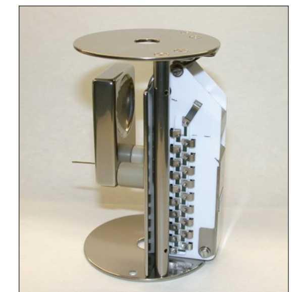
Figure 8. Photograph of a DM283 large-area HED detector.
